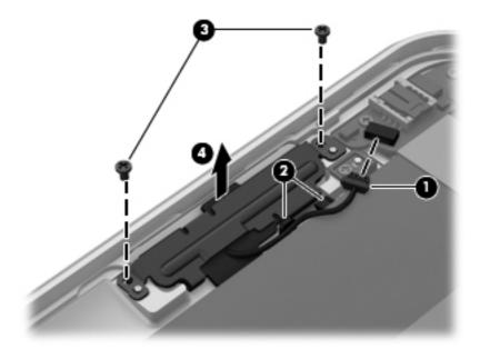
Reverse this procedure to install the volume button board.
